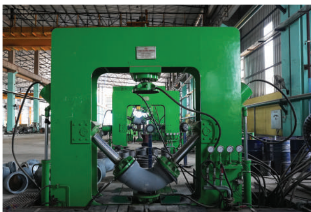
Hydrostatic Pressure Testing of Fittings
