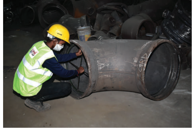
Inspection with Go, No-Go gauge
